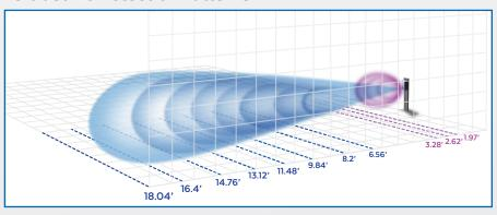
Microwave detection patterns (blue above) are adjustable from 6.56 to 18.04 feet. The Ultrasonic Sensor is for close range detection (purple). The OVS-01GT also features 5 sensitivity settings.
